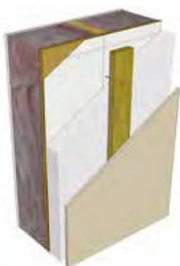
Screws through rigid exterior insulation
