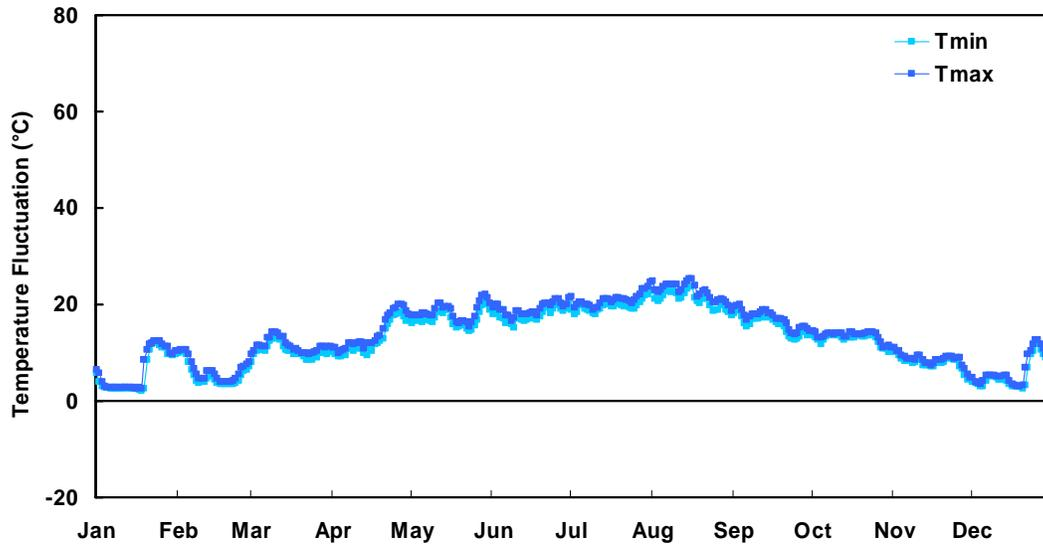
**Figure 17** The daily maximum and minimum membrane temperatures measured on Green Roof 2.
