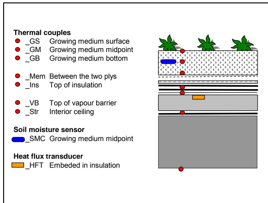
Figure 3 Cross-section of the BCIT Green Roof Research Facility's roofing system showing principal components and location of various sensors.
