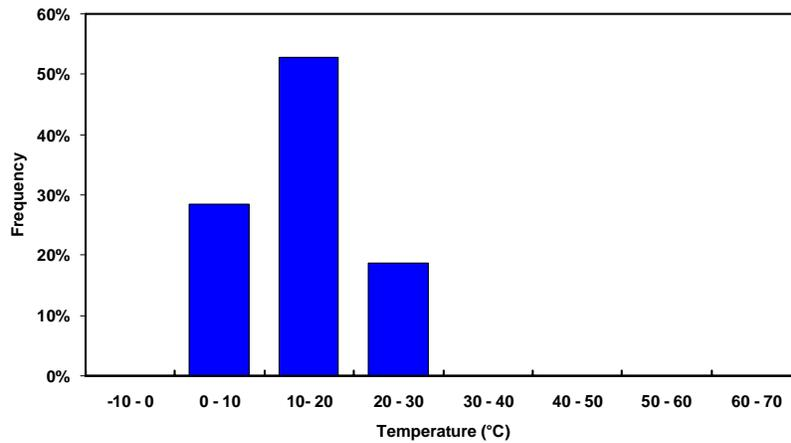
Figure 21 The maximum membrane temperature distribution of the three roof sections at the BCIT Green Roof Research Facility in 2005.
