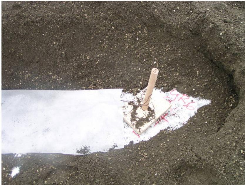
Photo 12 BCIT Green Roof Research Facility instrumentation test point; thermocouples installed in the growing medium.
