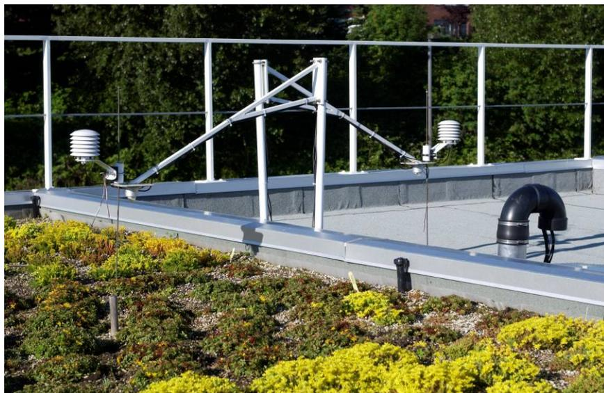
**Photo 14** BCIT Green Roof Research Facility weather pole, including solar radiation sensor, relative humidity and temperature transmitter, and thermocouples.
