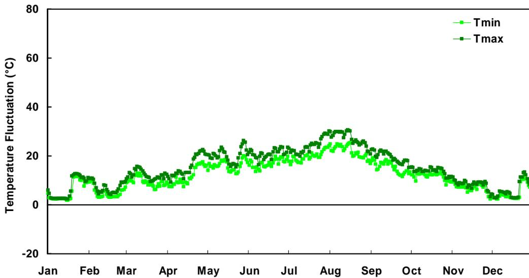
**Figure 16** The daily maximum and minimum membrane temperatures measured on Green Roof 1.
