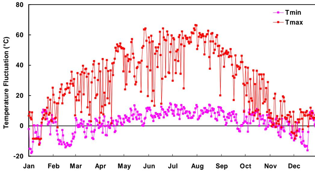
**Figure 15** The daily maximum and minimum membrane temperatures measured on the Reference Roof.
