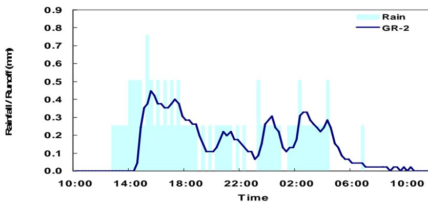
Figure 9 Reference roof and green roof runoff comparison during the April 5–6 rain event. 17.3 mm of rainfall were recorded over 18 hours.
