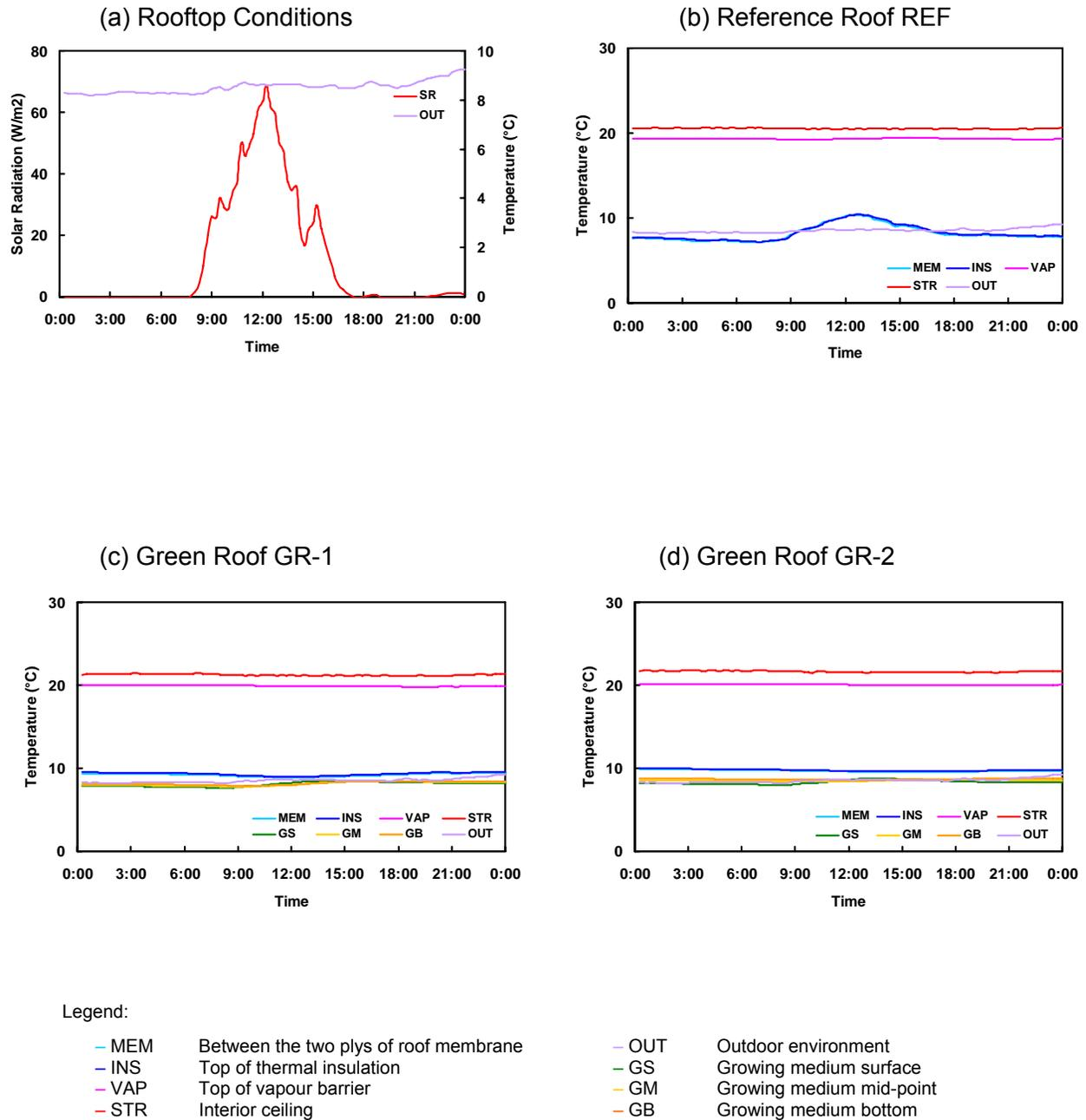
Figure 11 Weather conditions and temperature profile of the three roof sections at the BCIT Green Roof Research Facility on a typical winter day (January 30, 2005). Refer to Figure 3 for instrumentation location symbols.
