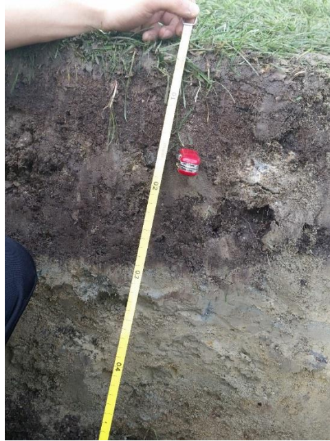
Figure 6. Upper part of a Factor 4 soil profile showing a dark colored Ap soil horizon overlying a lighter colored subsoil. 9
