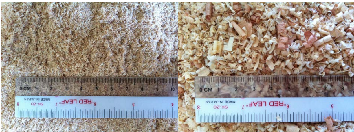
Figure 1: Fines. On a weight basis 50% of the fines are smaller than 2 mm, 50% shavings with a size of 4 to 25 mm
