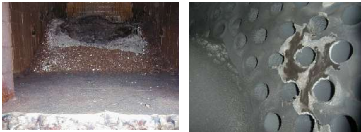
Figure 8: Example of clinker in a fixed grate combustor (left) and slag in a boiler (right)
