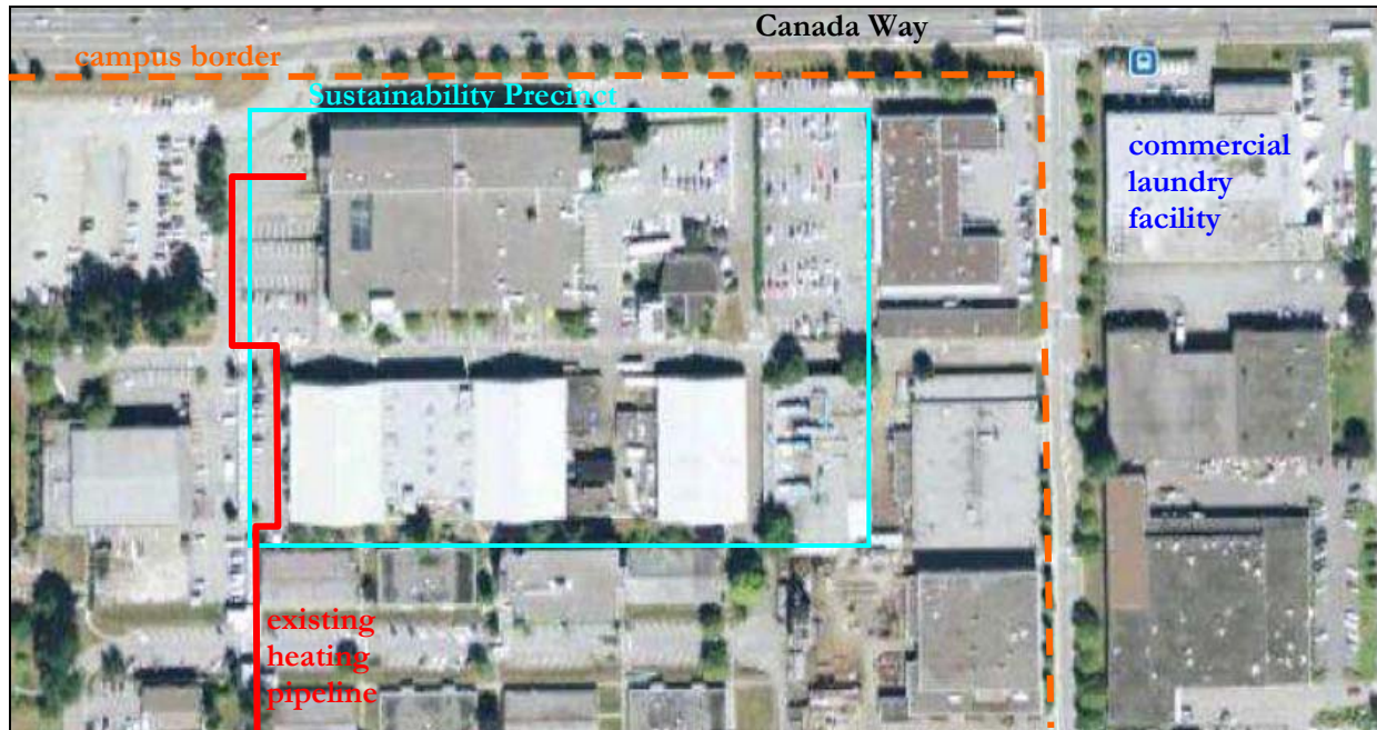
Figure 1.7 Location of a commercial laundry facility adjacent to BCIT's campus and in the vicinity of the Sustainability Precinct. The existing pipeline would have to be extended by approximately 400 m. Source of underlying satellite image: Google Earth.
