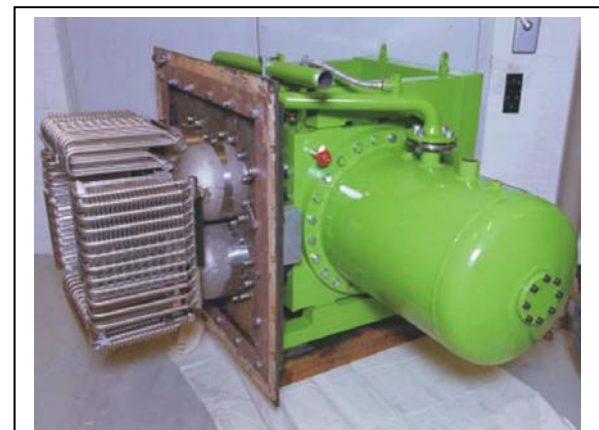
Figure 2.11 Sterling engine with a 35 kW electrical output. The heat exchanger on the left is inserted into the combustion chamber of a biomass boiler with a heat output of 250 kW, the size that is planned at BCIT's Joinery Workshop. Photo source: MAWERA Austria and Sterling Denmark.
