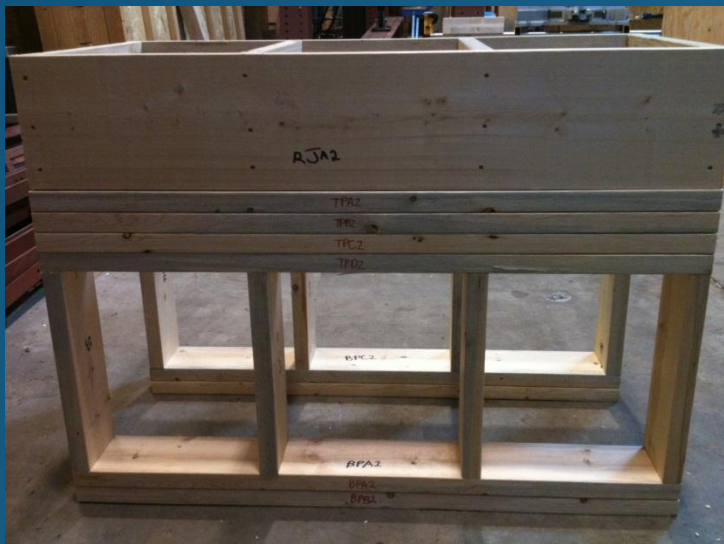
Figure 1. Small scale simulated wall/floor assembly under construction
