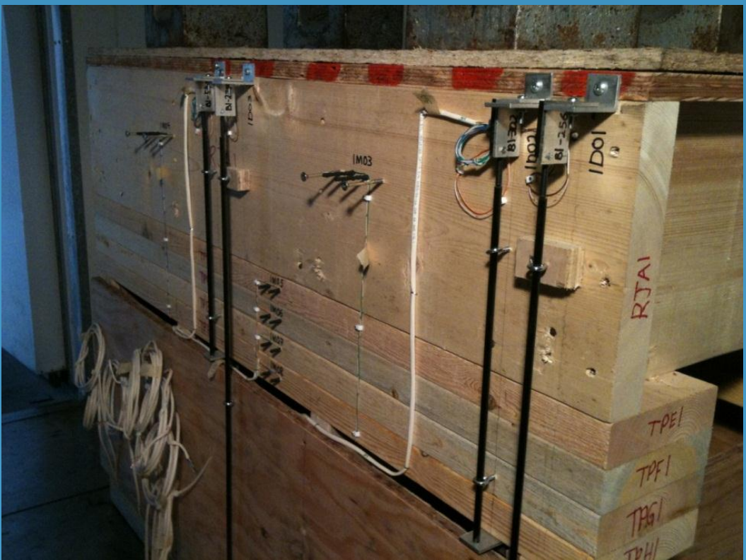
Figure 10. Displacement sensors and MC pins mounted on structure 1
