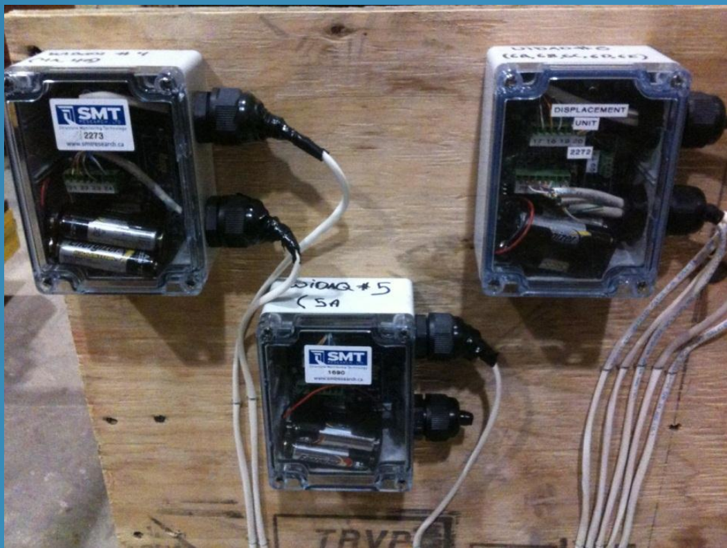
Figure 9. WiDAQs mounted on structure 2
