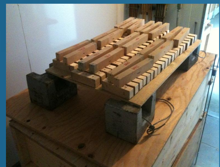
Figure 3. Sample blocks for assessing wood shrinkage coefficients being conditioned in a high humidity conditioning chamber
