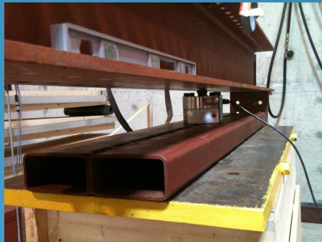
Figure 11. Load cell used to determine the load being applied by the lever arm system
