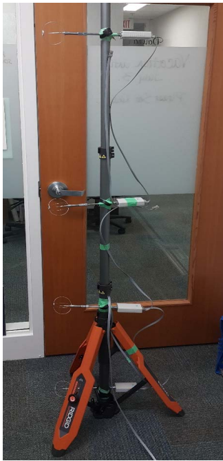
Figure 5 - Local Air Velocity and Temperature Measurement
